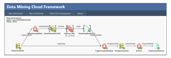
Fig. 3. Trajectories workflow at the end of the execution, with visualization of the final result.
